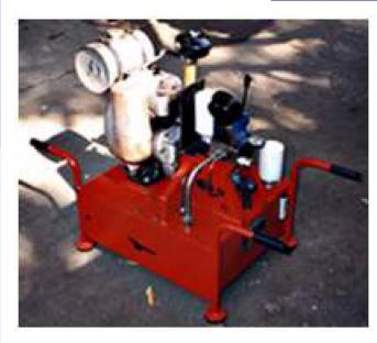
Pressure 700 bar Hydraulic power pack with electric motor / Diesel engine /Petrol engine driven are available with push button and lever operated directional control valves. Single stage construction available .Maximum discharge : 100 L/minMaximum working pressure: 700 bar.
