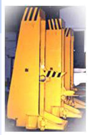
Electromechanical lifting jacks are used in sets for the lifting of Railway Rolling stock such as Engines, Bogies etc for repairing in Railway Workshops. They are also used for general repair work of big automotive jobs and wherever synchronous lifting is required.
