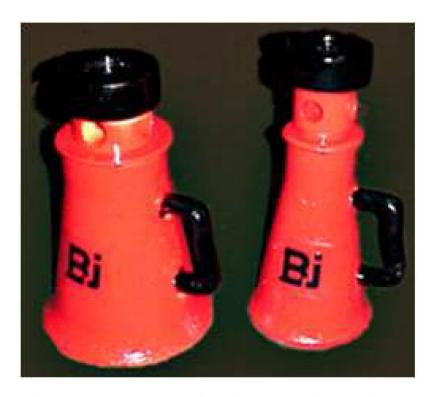
These are small height screw jack used for levelling of machinery & lifting of smaller loads. Its body is made of cast iron with hardened steel screw , bush & bearing as required.
